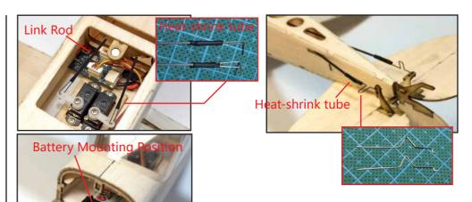
Adjust battery position front or back to adjust CG of this airplane.
