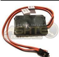
BEC is short for **Battery Eliminator Circuit** (UBEC = Universal BEC) (SBEC = Switching BEC). The BEC part of an ESC is completely separate from the circuitry which controls the speed of your electric motor.
