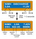
Set discharge current on the left and final voltage on the right. The discharge current ranges from 0.1 to 5.0A and the final voltage ranges from 0.1 to 25.0V). To start the process, press **Start /Enter** key more than 3 seconds.
