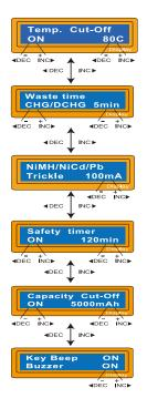
An optional feature using temperature probe contacting the surface of battery, the temperature cut-off can be on or off. If it is on, set the maximum temperature at which the charger should allow battery to reach during charge, Once a battery reaches this temperature during charge, the process will be terminated to protect the battery.
