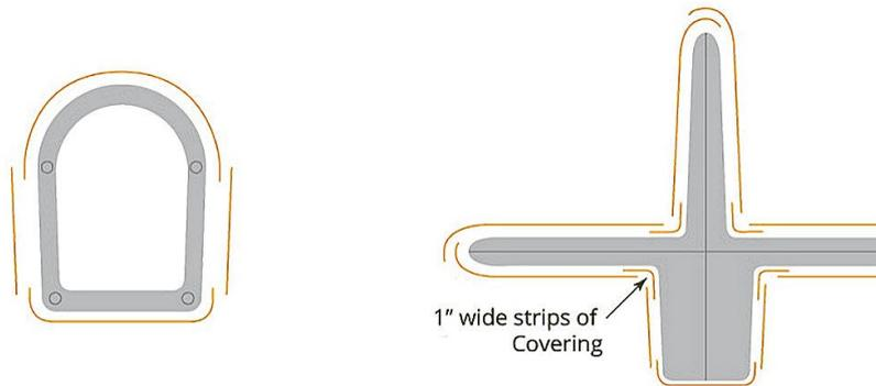
**Wings** - Cover each panel separately, with one piece of covering for the bottom panel first, and then another for the top panel.
