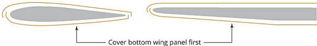
**Solid Surfaces** - Sheet balsa, ply. Cut the covering 1" oversize and place it on the required surface you wish to cover. Set the heat to LOW. Begin from the centre and iron outwards. Use light pressure to smooth the covering down, at the same time gripping the covering at the edge and pulling it outwards to stretch out any wrinkles and make it lie flat. Then iron that part down. It is important that you continue working outwards from the centre, until the entire surface is covered.
