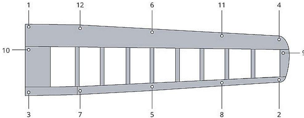
Now pull the covering gently to get a snug fit. If the covering produces large wrinkles then untack with the iron, pull gently to remove wrinkles and re-tack.
