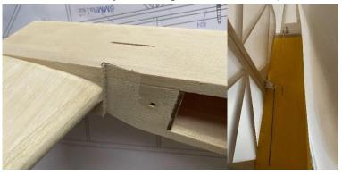
39-42 Use 8mm balsa sheets for the head section and 2pcs 8mm balsa sheets for bonding at the top.
