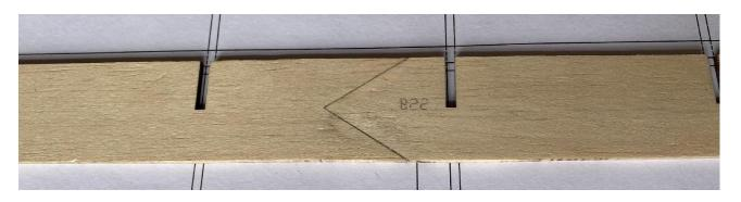
54-57 Install the wing ribs according to the drawing and paste 6X6mm balsa strips. The length of balsa strips shall be spliced.
