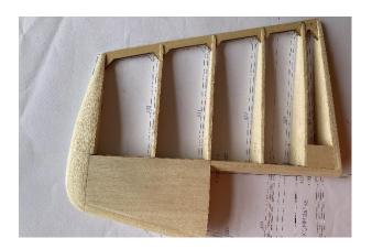
92-94 The horizontal tail is built according to the drawing, and 8mm balsa sheets are used for the reinforcement part.
