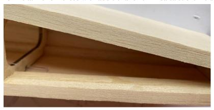
26-29 Tailplane was filled and glued with 8mm balsa sheets.
