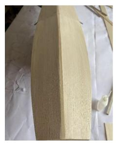
25 The tail is reinforced with additional 6X6mm balsa sticks inside.
