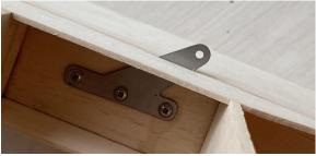
83-84 Drill 2.5mm holes in the 8X14mm pine strips and trim the strips to streamline.
