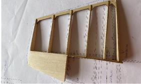
89-90 Glue 6mm balsa sheets on the front and sand them into a triangle shape. Glue balsa reinforcement blocks on the rudder corners.
