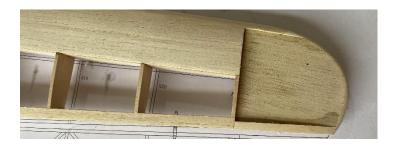
72-74 Assemble ailerons according to the drawings.
