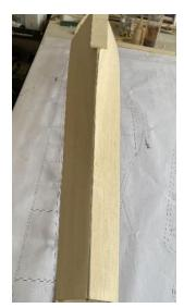
12 Sand the side cover and make sure it is perpendicular to the bulkheads.
