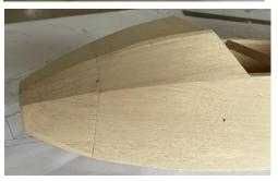
43-44 Steam 5X16mm pine sticks are heated for easy bending and forming.
