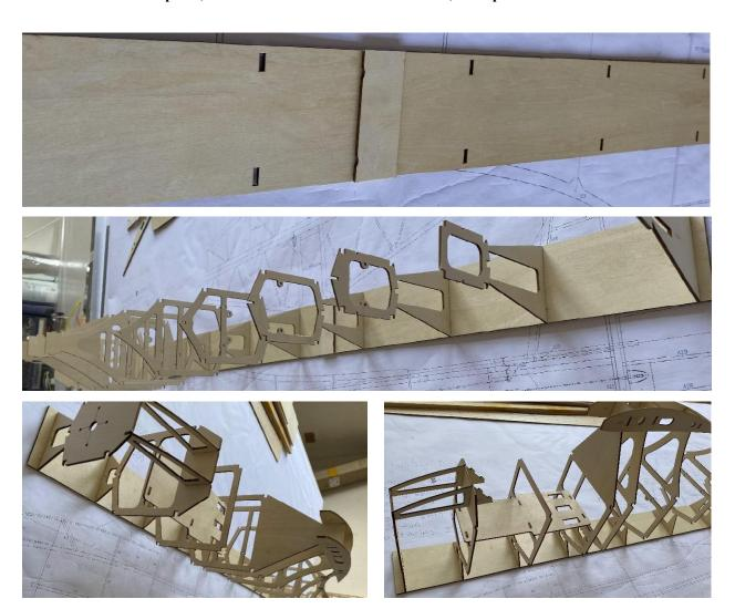
5-7 Wing platform cover plate of fuselage, cut out the line hole of aileron steering gear below, glue 8mm balsa sheet on the leading edge of the wing and sand it into shape, glue 6X6mm balsa to the bulkhead, use 6X6mm pine wood strips at the bottom front(for landing skid), and the rest are balsa wood strips.
