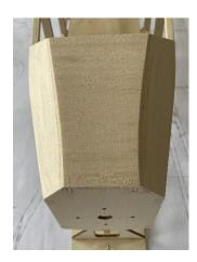
17 Reinforce the enclosure with pine stick. (It will have metal connectors at both ends to attach the wing struts) Note: The motor must be installed before pasting the mask; otherwise it is difficult to fix the motor with screws.
