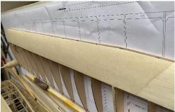
65-66 Glue 8mm balsa sheets on the leading edge of the wing and sand them into shape.
