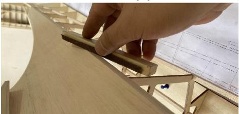
13 Attach magnets to A16 balsa for fixing the cabin cover.
