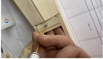
35-36 Mark the corresponding position of the PVC tube and cut out the pull rod hole.
