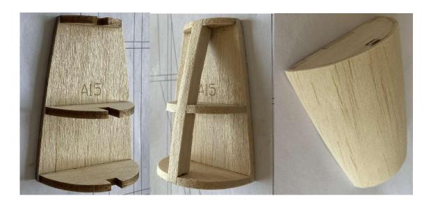
8. Make the leading edge of the wing table with two 5MM balsa sheets.
