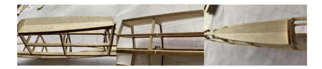
5. Make horizontal tail tiptable with 2 pieces of 5MM balsa sheets . You could use 5MM balsa sheet for positioning, glue and polish.
