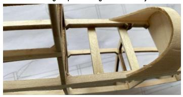
11. Glue the head cover in sequence (install the motor before attaching the head cover to the fuselage) and polish the shape.
