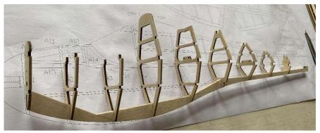
3. Glue the fuselage reinforcement strips.
